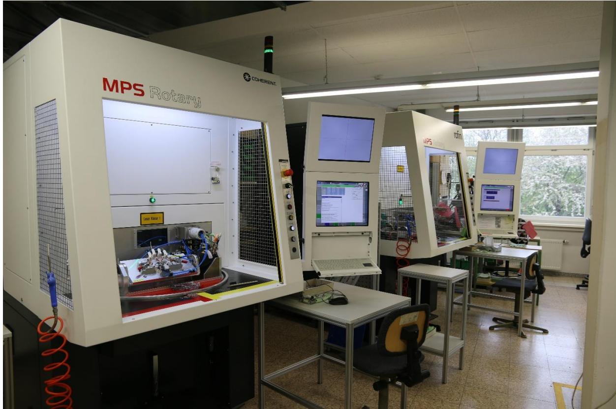
Figure 1: Two MPS Rotary systems for laser welding of glasses in the production at Silhouette in Linz, Austria
