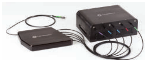
FIGURE 2. Multiple lasers can be integrated in a single Laserbox chassis, eliminating power supply and user interface redundancy; the fiber-coupled outputs can then be combined into one single-mode fiber using a plug-and-play beam combining module such as the Coherent Galaxy.
