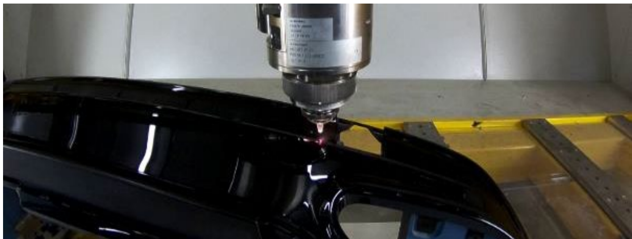
Cutting recesses for distance sensors and decorative strips using CO 2 laser
