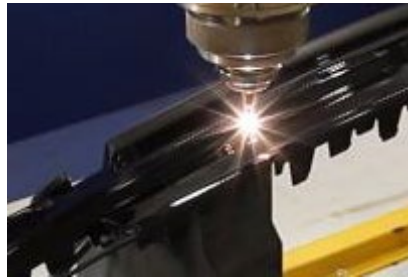
The CO 2 Slab laser ensures clean cut edges without burrs
