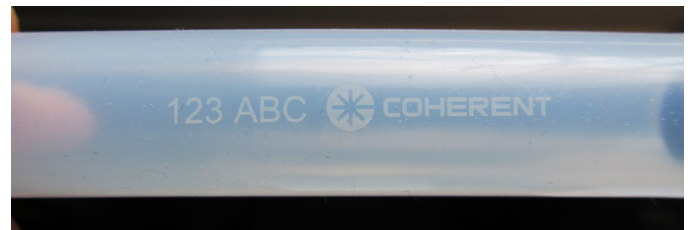
Figure 2. Ultraviolet lasers can mark colorless materials such as silicone rubber without affecting the outer surface.
