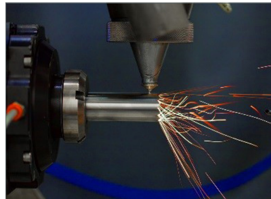
Figure 2. Laser cutting of a TAVR aortic valve out of a metal tube (e.g. nitinol).
