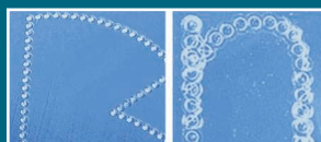
► Figure 2: Engravings in mineral glass using the 193 nm Excistar laser at a spot size of 40 μm (left image) and a q-switched pulsed CO 2 laser at a spot size of 120 μm. The CO 2 laser mark shows thermal effects due to the longer wavelength, including uncontrollable microcracking. ►
