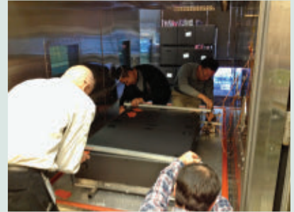
FIGURE 3. A key part of delivering industrial-grade reliability is HASS testing. Here, technicians at Coherent strap down a laser to a vibration table inside an environmental test chamber prior to subjecting the laser to comprehensive “shake and bake” testing.
