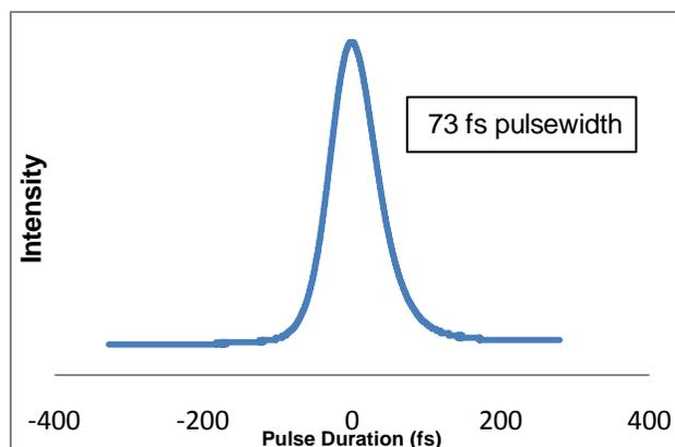
**Figure 2**, Autocorrelator trace showing 73 fs pulsewidth
