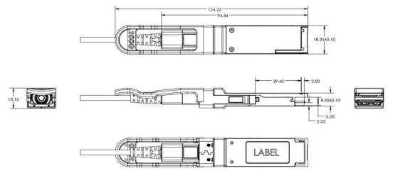
Figure 2. Module Mechanical Dimensions
