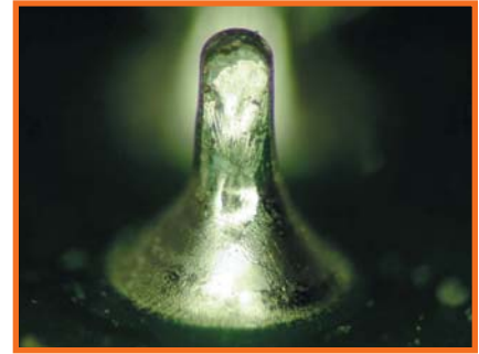
FIGURE 3: Optimized joint; Sn-Ag solder, 10W. 0.8 sec.
