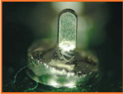
FIGURE 1: Severe dry joint; Sn-Ag solder, 6W. 0.8 sec.
