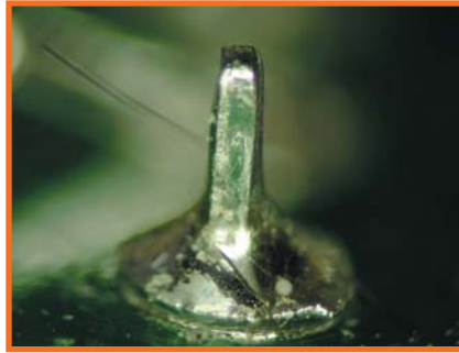
FIGURE 2: Dry joint; Sn-Ag solder, 8W. 0.8 sec.
