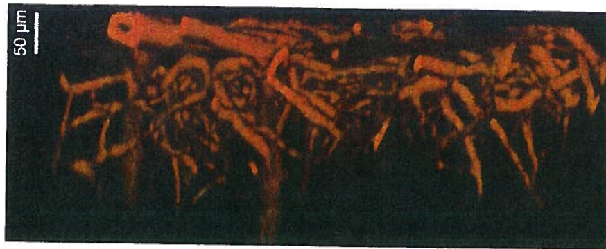
Figure 3. Long-wavelength excitation is critical for deep-tissue imaging, as illustrated by this image of mouse brain capillaries extending to a depth of 250 \mu\text{m} . The image was recorded with 1080-nm excitation using an Olympus objective and Coherent Chameleon Vision. Courtesy of Dr. Hiroyuki Kawano, Professor Atsushi Miyawaki Lab, Laboratory for Cell Function Dynamics, Brain Science Institute, Riken Institute, Japan.
