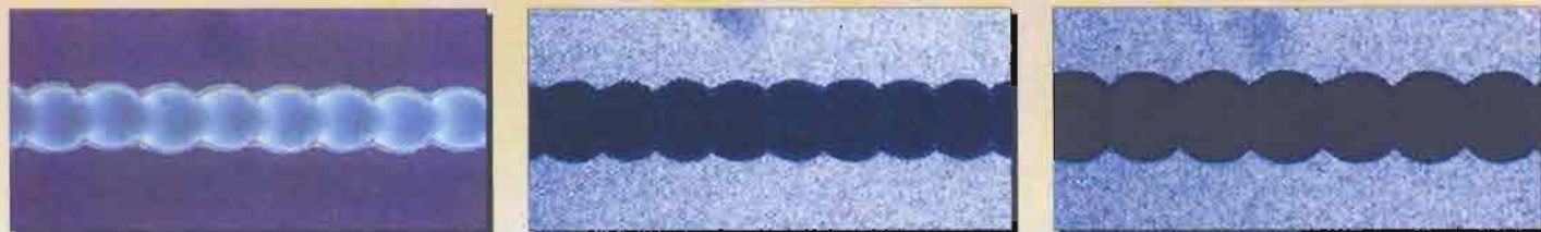
6. Prisma lasers use a high pulse repetition frequency (PRF) to achieve the desired scalloped profile in scribing. The scan rate is >2 m/sec.
