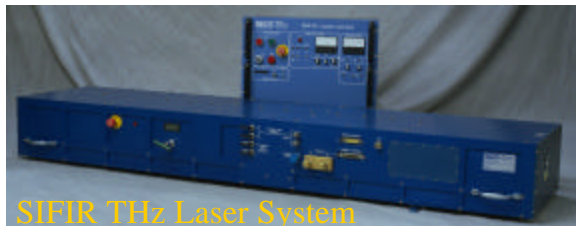
Figure 22: Photograph of the Coherent-DEOS SIFIR-50 OPTL. This laser is going to be used as the LO for a THz receiver at the AST/RO facility at the South Pole.
