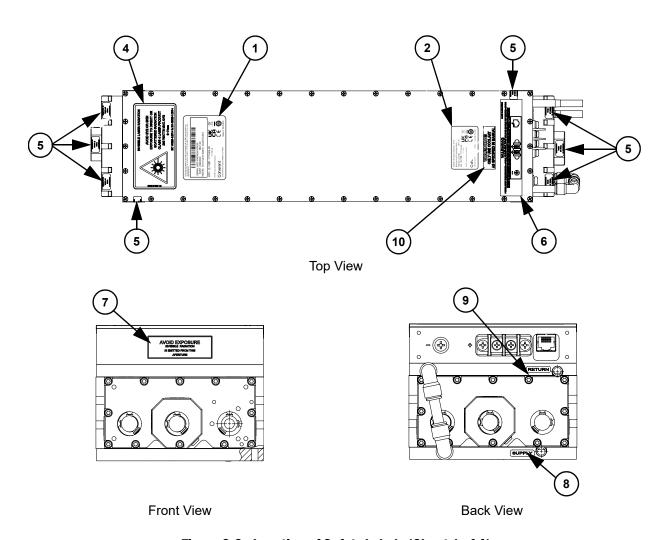
Figure 2-2. Location of Safety Labels (Sheet 1 of 4)
