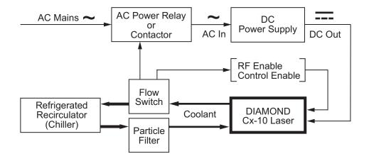
Figure 4-3. Recommended Liquid Cooling System Functional Block Diagram
