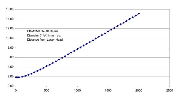
Figure 4-7. Beam Diameter vs. Distance From Laser Head
