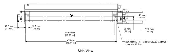
Figure 4-2. Cx-10 Liquid-Cooled Laser Dimensions
