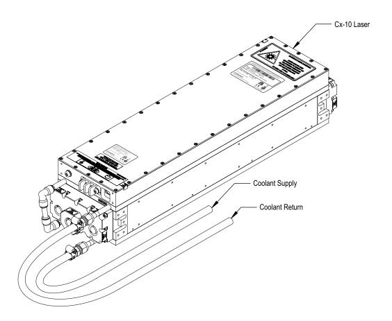
Figure 4-4. Cx-10 Liquid Cooling Connections
