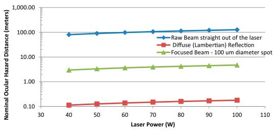
Figure 2-1. Nominal Ocular Hazard Distance (NOHD) for indicated conditions calculated per ANSI Z136.1-2007
