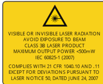
Figure 2.4-1: IEC-style Classification / Warning Logotype, and Manufacturer / Product-info Label, and location-illustration of Left-side (facing the Front Panel) of the unit.
