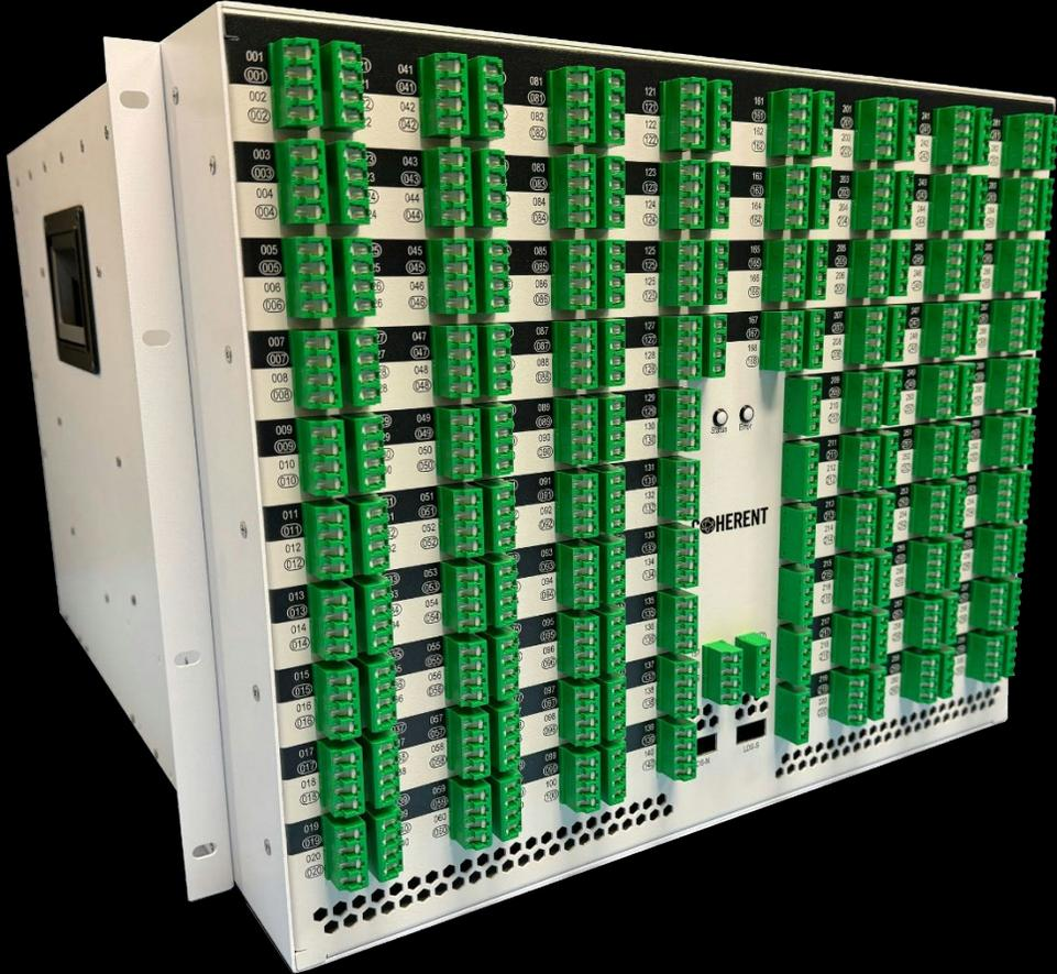
Coherent Datacenter Lightwave Cross-Connect (DLX™)
