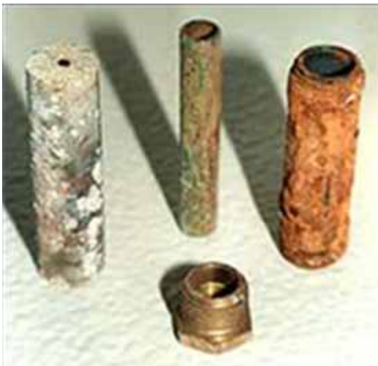
Untreated Water Circuit
