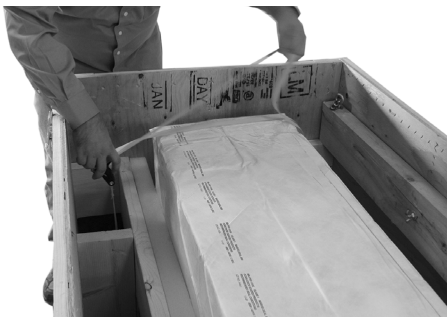
Figure 4-10. Unstrapping the System
