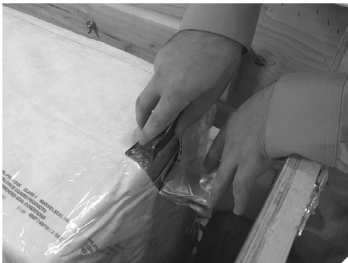
Figure 4-11. Exposing the Eye-bolt Holes
